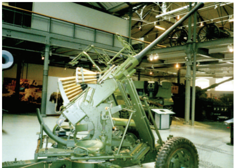
A towed 40mm Bofors Gun: The classic light anti-aircraft weapon
